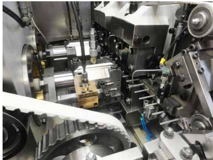
Fig. 2: Positioning of the pins in the transport belts. First and second punching stations
