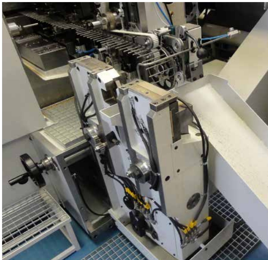
Fig. 4: Multicutting unit for straight cut or for self-drilling points, diamond points etc.
