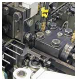
▲ Holding the wire nail blanks with clamping jaws and upsetting the nail head
